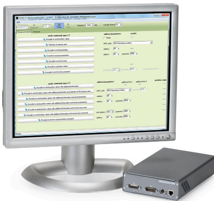
Figure 1: PWM 21 with the EnDat 2.2 Demotool software
